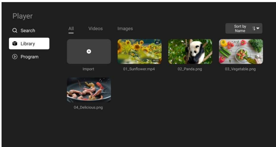
Step 3 To import new media files, select **Import**, select a file, and then press the **Confirm** button on the remote.
