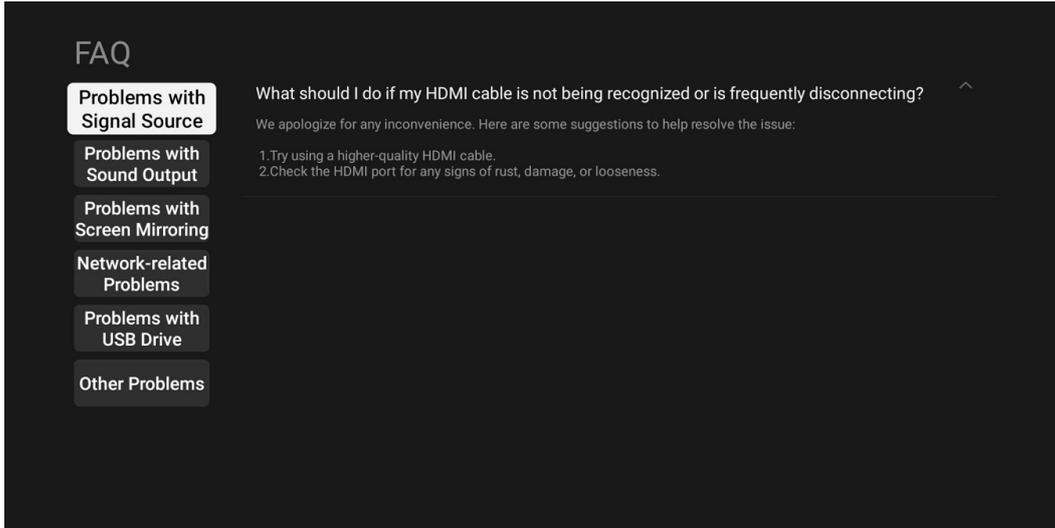
Step 2 Use the remote's **Up** and **Down** buttons to toggle between the categories of issues on the left, then press the **Confirm** button to view the specific questions.
